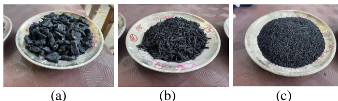
Figure 1: Rubber particle sizes (a) 10-20mm, (b) 5-10mm, (c) 0-5mm.
