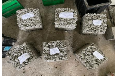
Figure 7: Casted porous concrete cubes.
