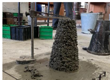
Figure 8: No slump concretes.
