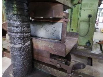
Figure 4: Splitting tensile test setup.
