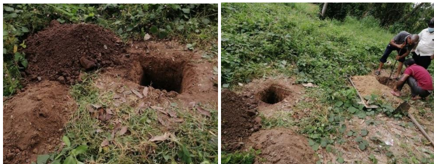
Figure 5- Percolation Test Pit 1 and Pit 2.
