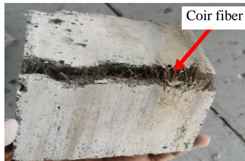
Figure 3.2: Distribution of coir fibers in AAC material.
