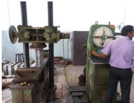
Figure 5: Loading prisms by AMSLER testing machine.
