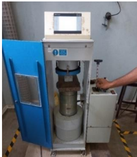
Figure 4: Crushing mortar cubes using a universal testing machine (UTM).
