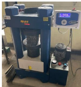
Figure 6: ASTM C39 Standard Compressive Strength Test.
