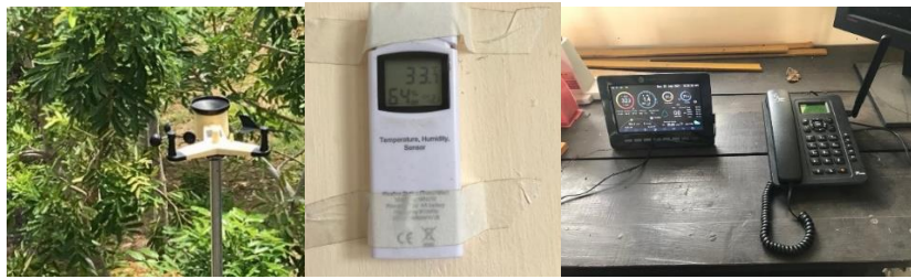
Figure 2: Instruments to be used in this field study; (a) Ambient Weather WS-2000 OSPREY Weather Station (b) Thermo-hygrometer sensor (c) Datalogger.
