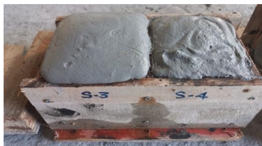
Figure 3.1: Casting fiber-reinforced AAC cubes.
