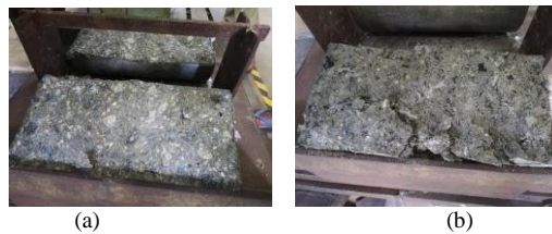
Figure 5: After the failure of cylinders (a) NC, (b) RuC.
