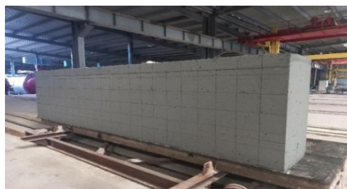
Figure 2.3: AAC cube before steam curing.
