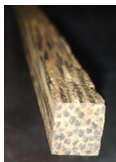
Figure 8: Kithul wood rebar 10\text{ mm} \times 10\text{ mm} square section.
